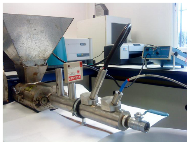
Fig. 1. System designed for this work in order to take Raman measurements.
